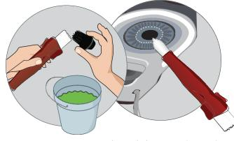
Remove nozzle and clean. Soak nozzle in sanitizer solution for no more than 5 minutes. Scrub injector ring with sanitizer and brush, then repeat. Allow to air dry for 2 minutes.
