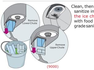
Remove upper and lower ice chute inserts. Clean, then soak in sanitizer for two minutes. Air dry then reinstall ice chute inserts.
