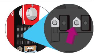
Clean cartridge probes until the cloth comes away clean. Repeat. Then allow to air dry for 2 minutes.
